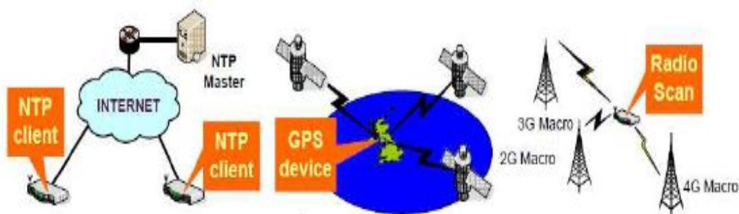
Figure 5.1.3: Femtocell current synchronization solutions
