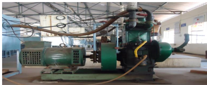
Fig.5 Photograph of Experimental engine and alternator.
