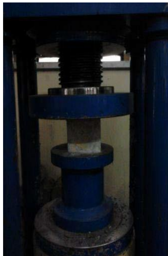
Figure 3. Testing of cube in compression testing machine after 28days curing.
