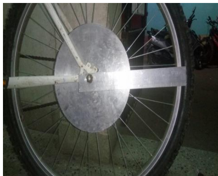
Figure 3: Implemented setup of eddy current brake
