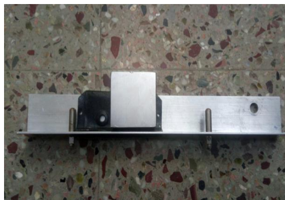
Figure 2: Magnet attached in the sliding frame
