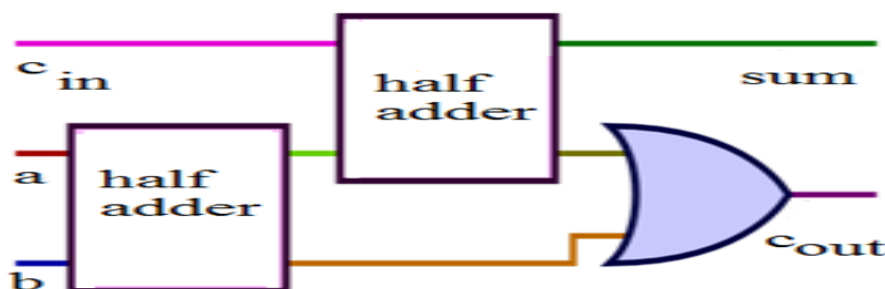
Fig 3.Full adder using half adder
