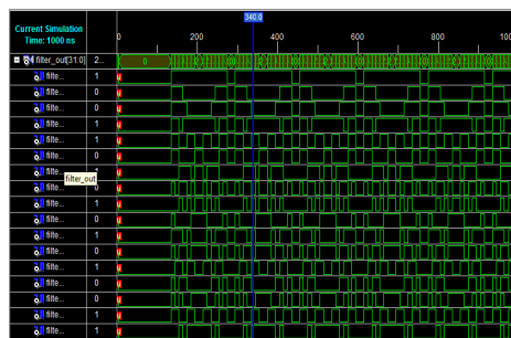
Fig. 12 Output of direct form FIR filter
