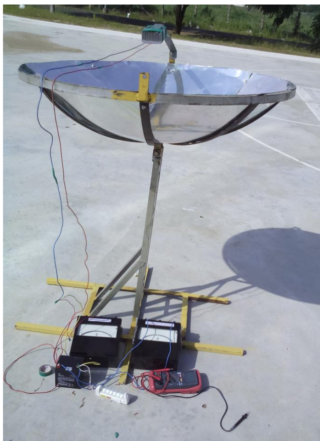
Figure 1: The arrangement of TEG setup with parabolic reflector
