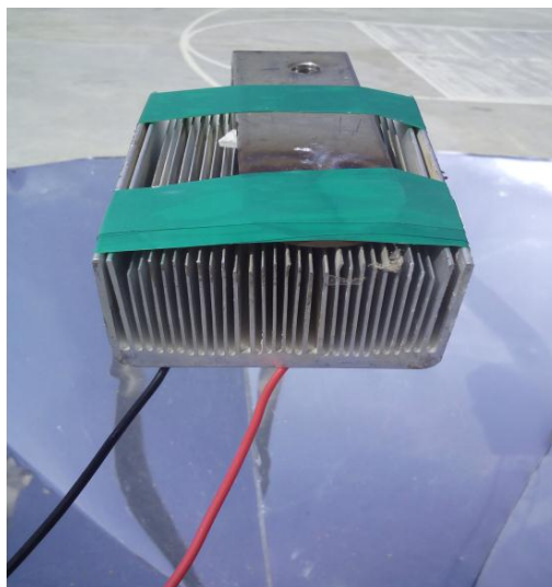
Figure 21 TEG setup below the heat sink
