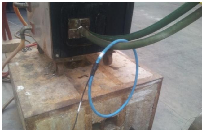
Fig.12 Application of rogowski coil for induction heating
