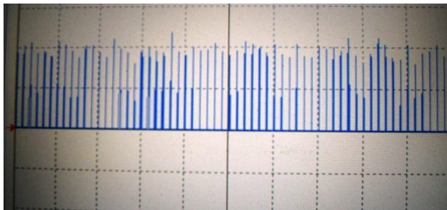
Fig4 .screen shot of gate pulses applied to gate-source terminal of the MOSFET switch
