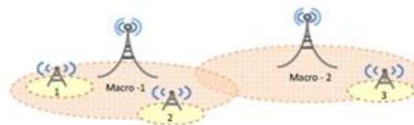
Figure 2 HETNET architecture - low power node 1 is used capacity improvement in a hot-spot; low power node-2 and low power node-3 are used for improving edge throughput
