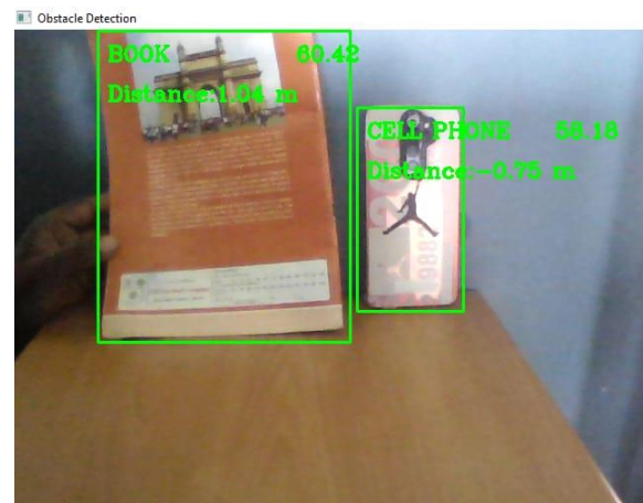
Fig 8.2 Multiple Objects detection with distance
