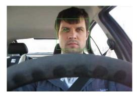
An eye tracker is a device for measuring eye positions and eye movements. Eye trackers are used in research on the visual system, in psychology, in marketing, as an input device for human computer interaction, and in product design.
