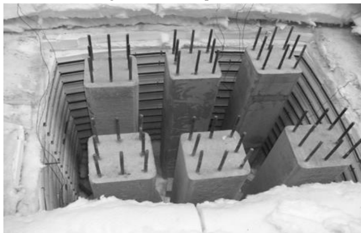
FIG. ARRANGEMENT OF POST-HEATED SQUARE REINFORCED CONCRETE COLUMNS IN FURNACE
