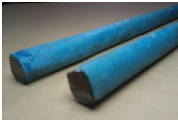
Side view of coated rebar
