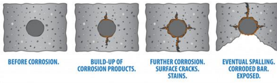
Fig 1.1 Corrosion Mechanism in concrete
