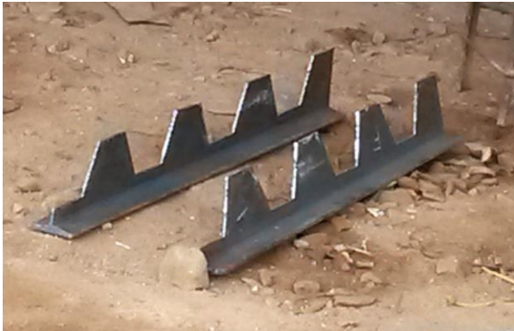
Fig 5: I beam after gas cutting
