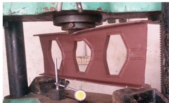
Fig 9: Deformed specimen(Litzka beam with stiffeners)
