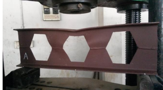
Fig 7: Deformed specimen (CSB)
